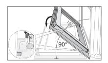
4. Fold up the clamping levers (A) on both door hinges back into their original positions.
